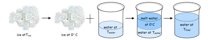
a) Get an ice cube, find its mass and note the temperature in the cooler:
