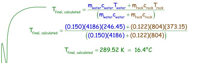
f) Report your measured and calculated final temperatures and reflect on them. How close are they? Did the specific heat of water compared to the rock's show up as a significant effect in this experiment? Think about what the result would have been if you dropped water of the mass and temperature of your rock into the cold water.
