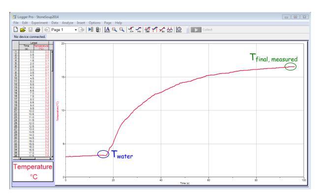
c) Record the temperature of the water just before the rock was dropped in and the final temperature of the mixture as the curve flattens out (it will keep warming slowly due to the heat in the room)
